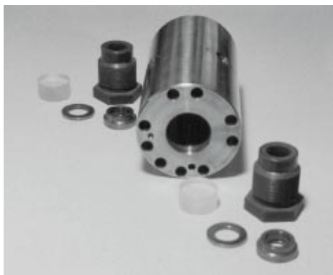
Figure 2. Optical cell with seals and sapphire windows for the measurement of phase boundary lines and densities in SCW. See text for details.
